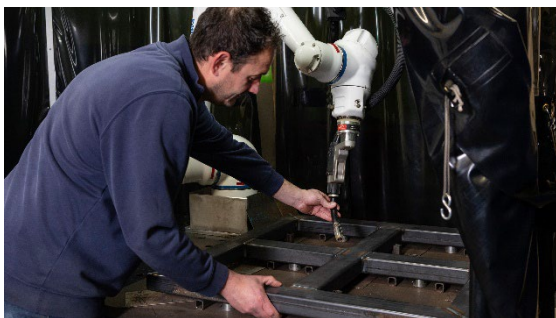
Cobot welding application. Picture Source: Yaskawa
