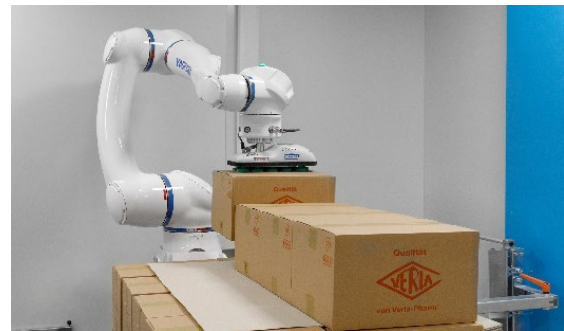
Palletizing cobot. Picture Source: Yaskawa.
