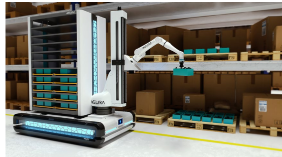
Mobile manipulator palletizing products. Picture Source: Neura Robotics.
