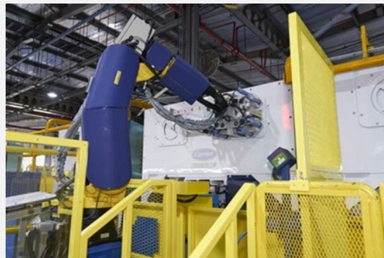
Robot mounting refrigerator doors. Picture Source: Touché Solutions
