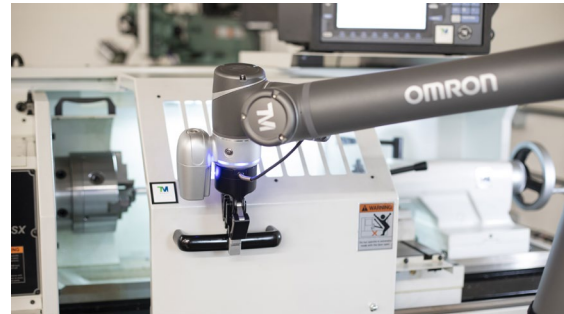
Cobots can work side-by-side with humans in many applications, e.g. closing a CNC machine. Picture Source: OMRON.
